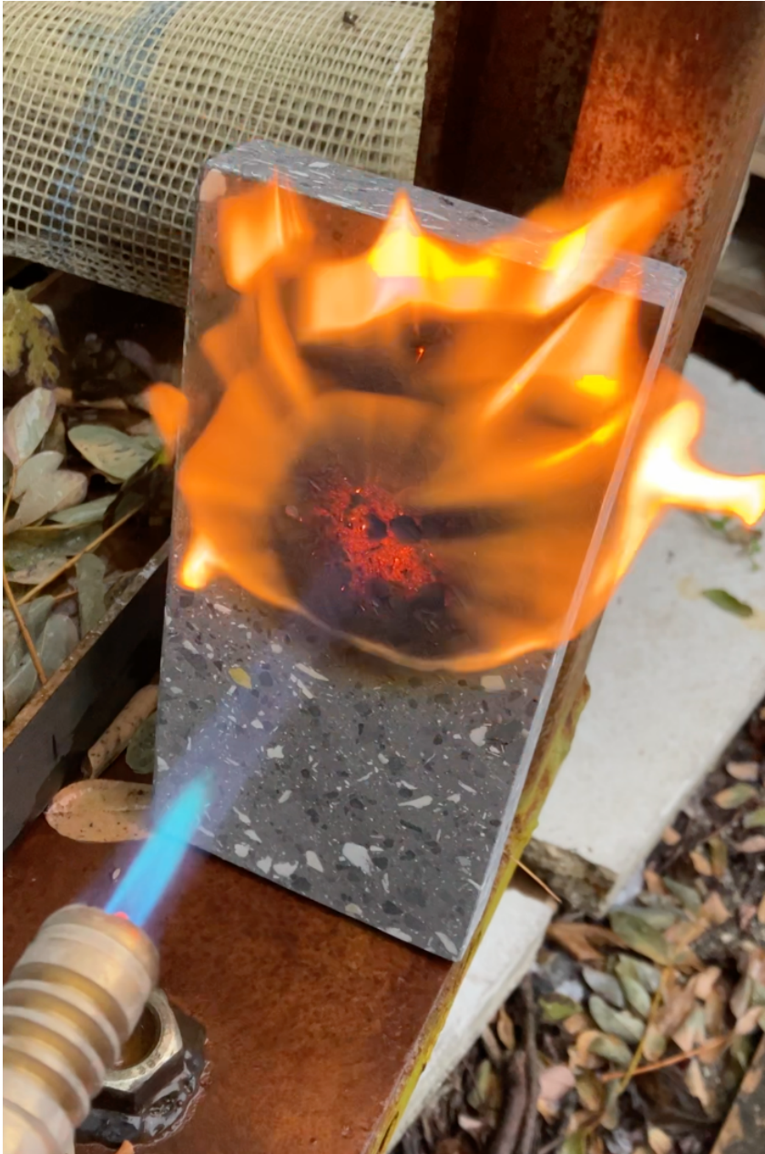
Picture 7. Flame behaviour tests following EN 13501 FL
