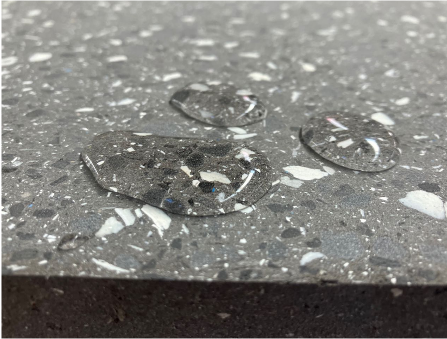
Picture 5. Hydrophobic behaviour of test 104.45
