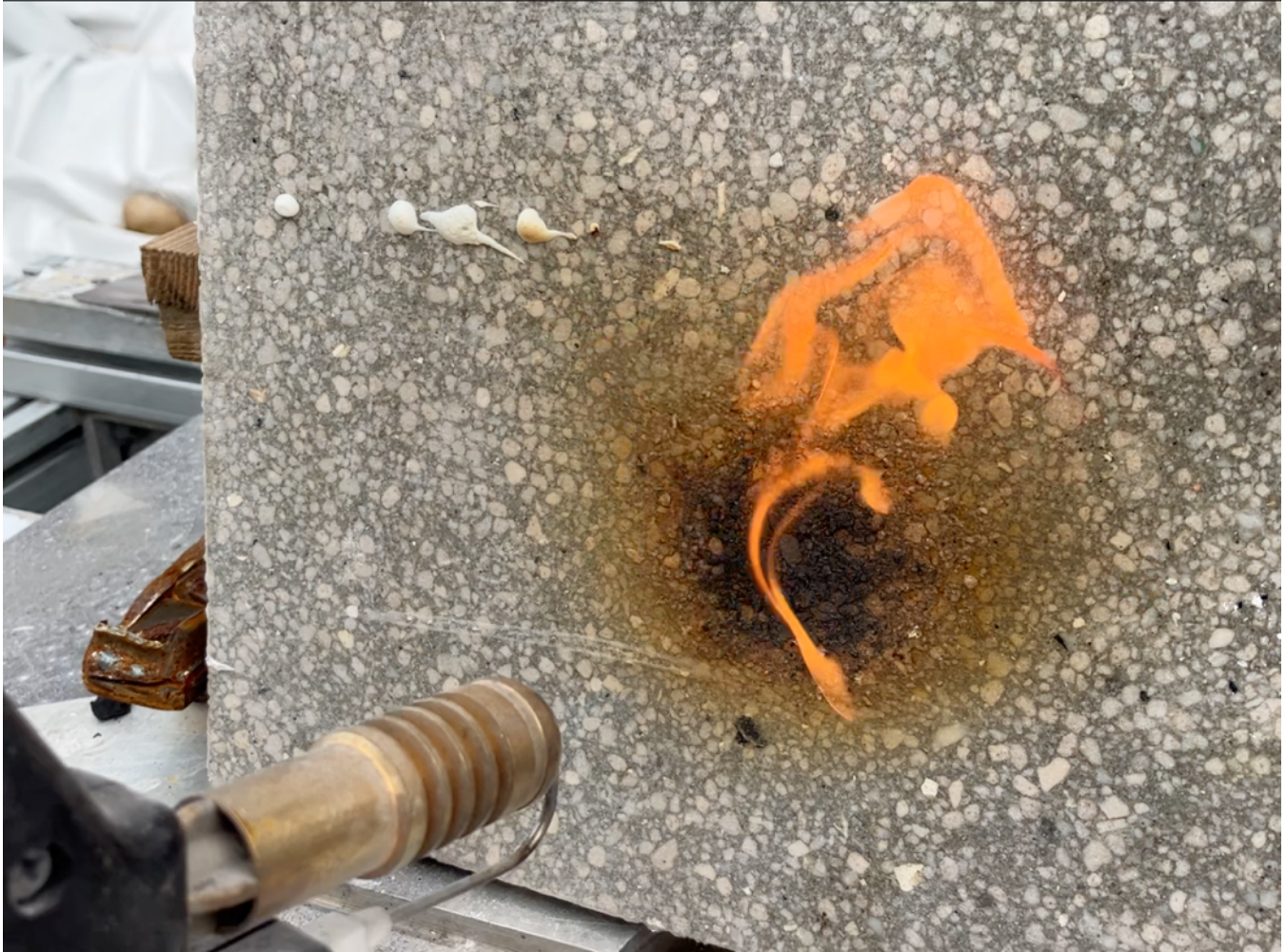
Picture 5: Flame behaviour tests following EN 13501 FL
