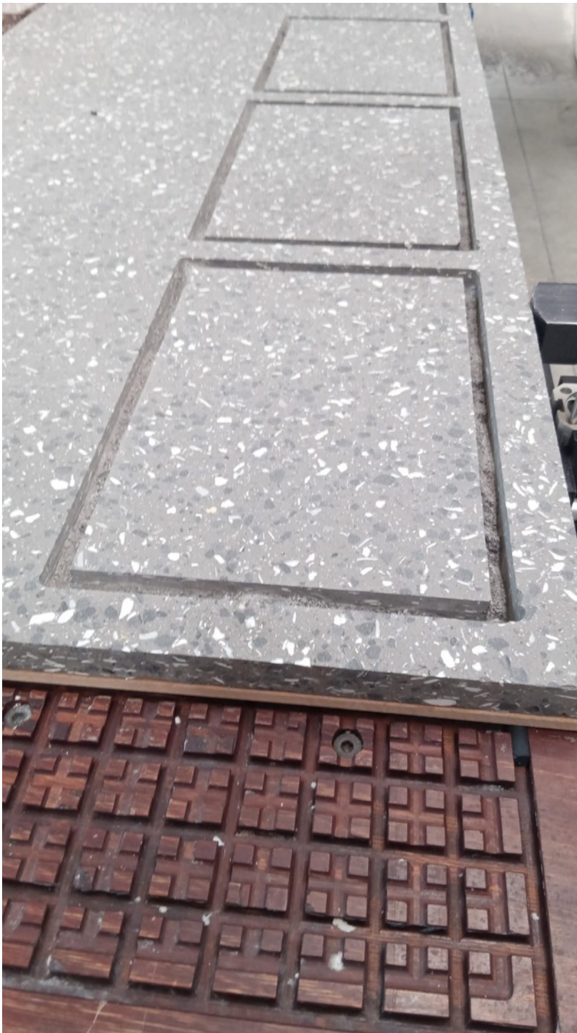
Picture 7: CNC milling of Type 2 panel coated
