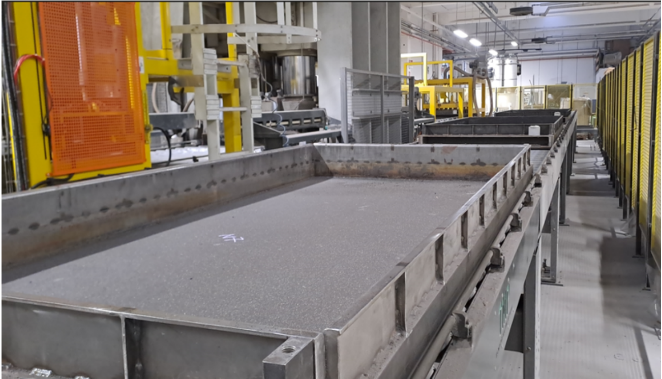
Picture 13: Panel on production line
