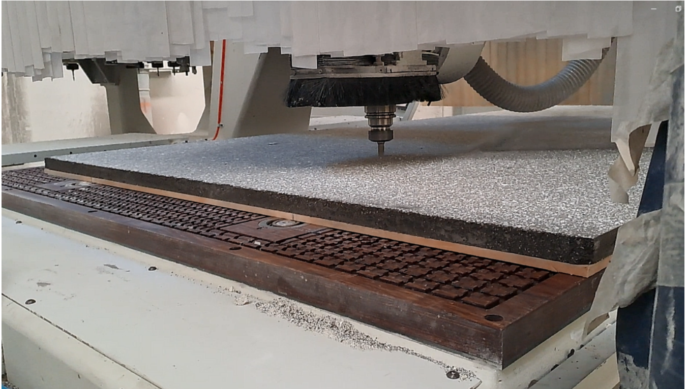
Picture 6: CNC milling of Type 2 panel
